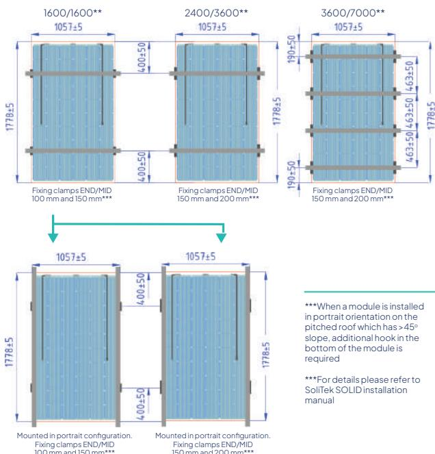
\*\*\*When a module is installed in portrait orientation on the pitched roof which has >45° slope, additional hook in the bottom of the module is required
